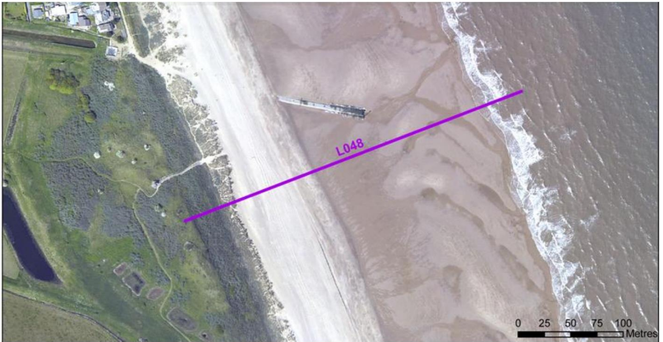
Plate 7.8 Aerial photograph of the beach at transect L048 (see Figure 7.16), showing outfall and wet sand with channels running out to sea on the lower beach. Photo from 26 May 2012 (Environment Agency, 2013a). Transect is located in the northern half of the offshore ECC.
